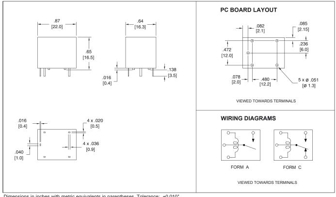
Dimensions in inches with metric equivalents in parentheses. Tolerance:  $\pm 0.010$ "
